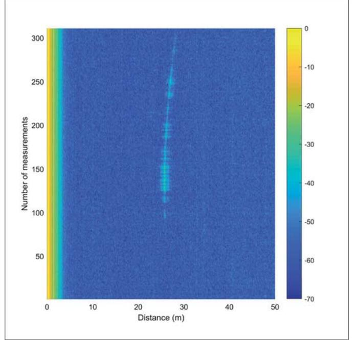
Fig. 4. Radargram for the detection of the bird shown in Fig. 3.
