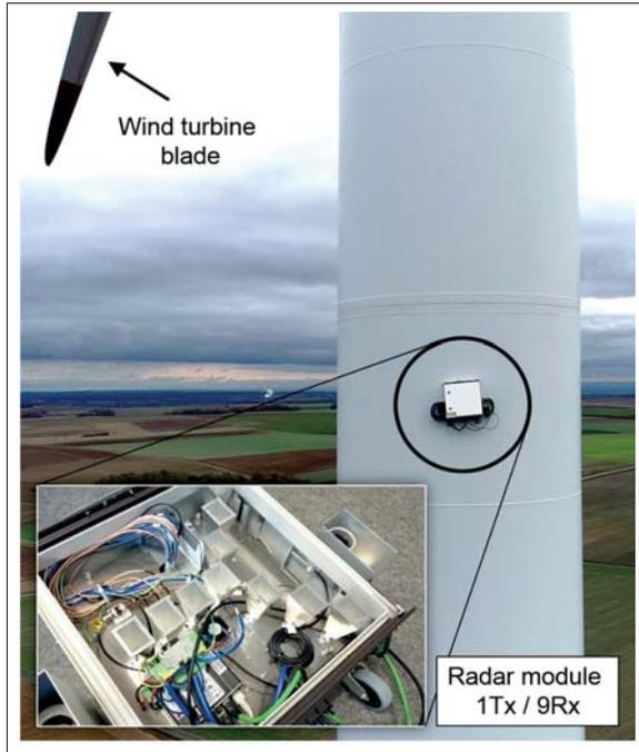
Fig. 1. Radar system installed at the tower of a 2MW wind energy plant about 95 m above ground. The FMCW radar operates in Ka-band from 33.4 GHz to 36.0 GHz and consists of one Tx and nine Rx-modules.
