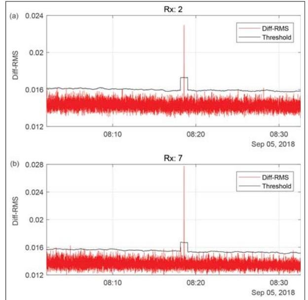
Fig. 2. Diff-RMS for two radar channels (a) Rx: 2 and (b) Rx: 7. The peaks in both curves indicates that both radar receivers were able to detect the bird event independently and automatically.
