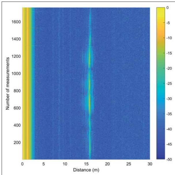
Fig. 6. Radargram for the detection of a drone where the drone moves approximately 16 m in front of the radar.
