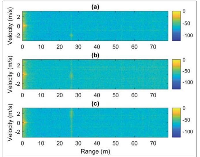
Fig. 5. Range-Doppler map of a bird: (a) target is moving towards the radar. (b) target is located in front of the radar and has no radial velocity, and (c) target is moving away.
